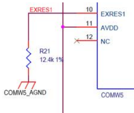
Figure 2. External reference resistor
